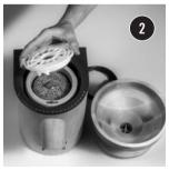
You can now lift the upper stone (stator) and control the milling surfaces.
